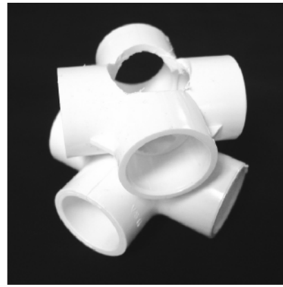
B. Stack of crosses. Partially drilled and through-drilled cross, rotated 45° ready for placement of pole
